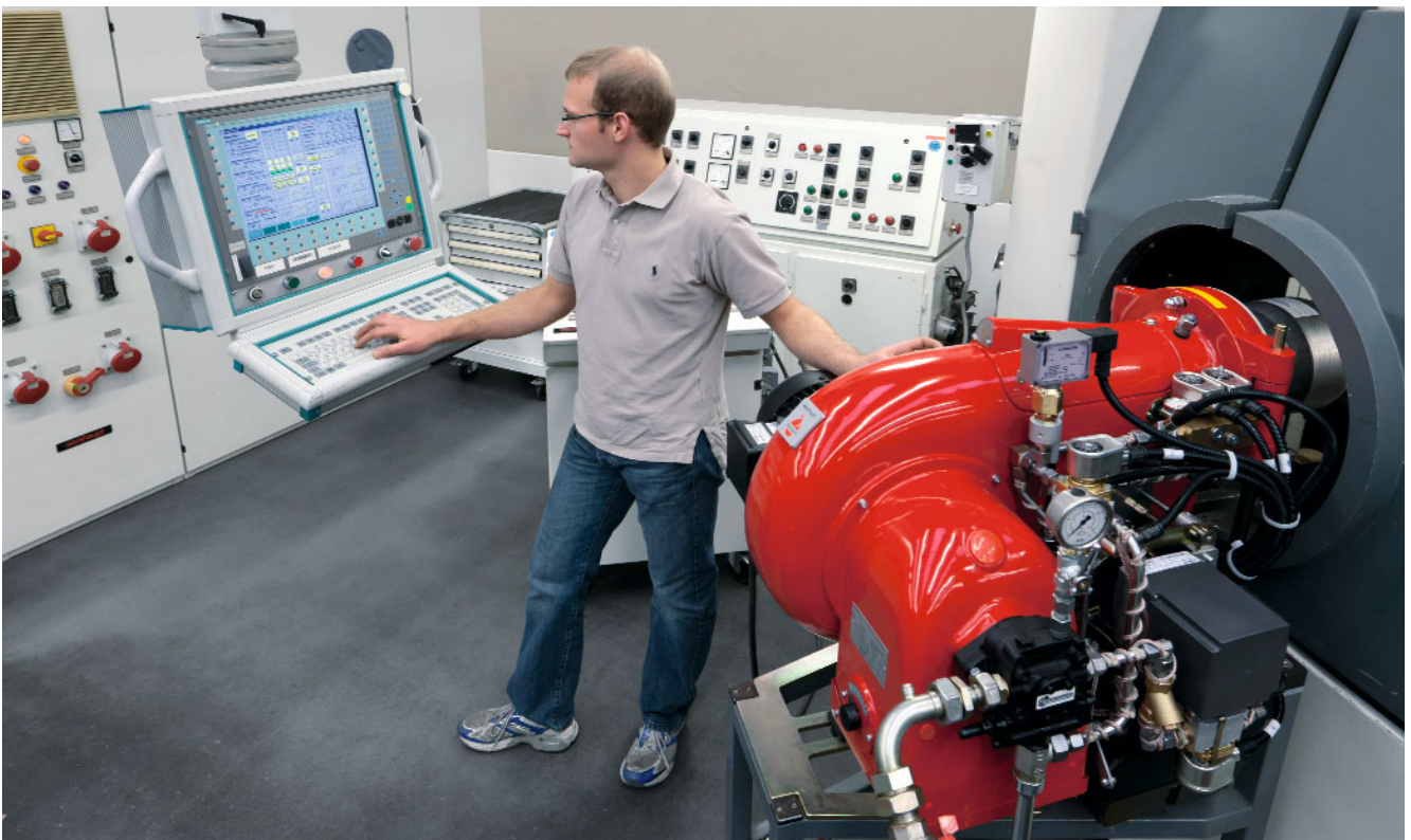
All burners in marine execution are fully tested on special test beds prior to delivery
